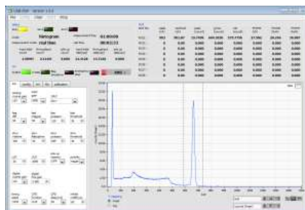
LaBr3(Ce) detector and using Cs-137 radiation source (Peak spectra of γ-ray @662keV and Ba-Kα ray @30keV)
