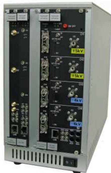
Positron Lifetime Measurement System (From the left sequentially: 3G ADC, 100M ADC, Preamp power supply, High-voltage power supply)
