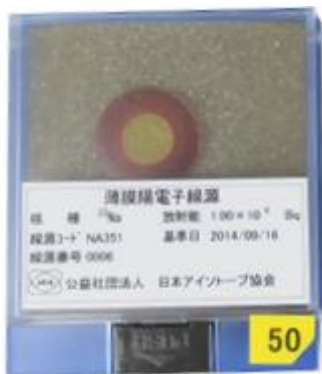
Photo 3. Thin film positron source Na-22
