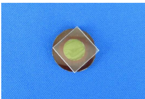
Photo 4. Figure sandwiching the source with reference material (photographed from above)
