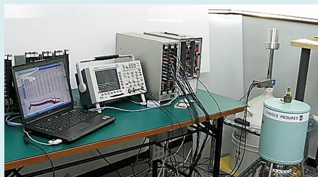
We are testing and inspecting using Ge semiconductor detector and Si (Li) semiconductor detector owned by our company.
