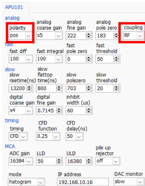
Since the detector's signal polarity has been confirmed as positive on the oscilloscope, set the "polarity" to "pos" in the application. Additionally, since the preamp output type is resistive feedback, set the "coupling" to "RF".
