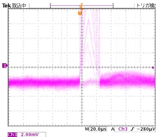
Adjusting the "slow pole zero" to 708 digits completely eliminated the undershoot, confirming that the adjustment was successfully made.
