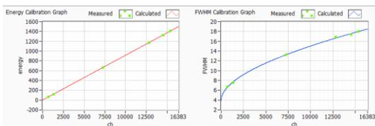
Based on the selected ROIs, energy calibration and FWHM calibration are calculated instantly, and the result graph is displayed.
