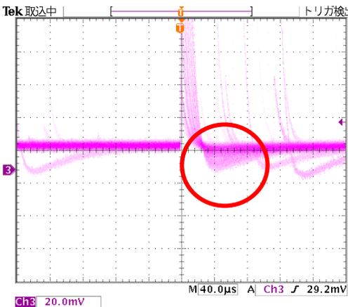
Upon checking the oscilloscope, it was observed that the waveform undershoots after the falling edge.
