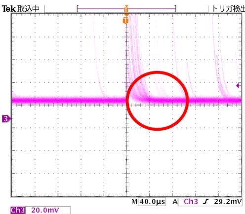
By increasing the value of "analog pole zero," the overshoot has been eliminated. The current "analog pole zero" value is 190 digits.
