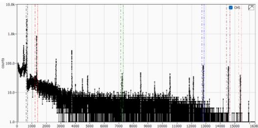
After entering the values for ROI start and ROI end, the spectrum will display the vertical lines at these points, as shown in the image.
