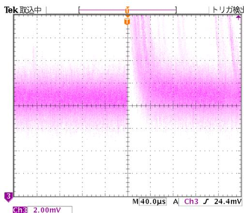
When the voltage range was changed from 20mV to 2mV, a slight overshoot was still observed.
