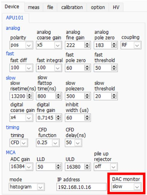
In the application, select the "slow" monitor signal type. The waveform type of the monitor output will switch to the fast signal.
