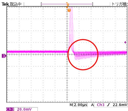
This is the oscilloscope image of the fast signal before adjustment. It can be seen that there is an undershoot after the waveform's falling edge.
