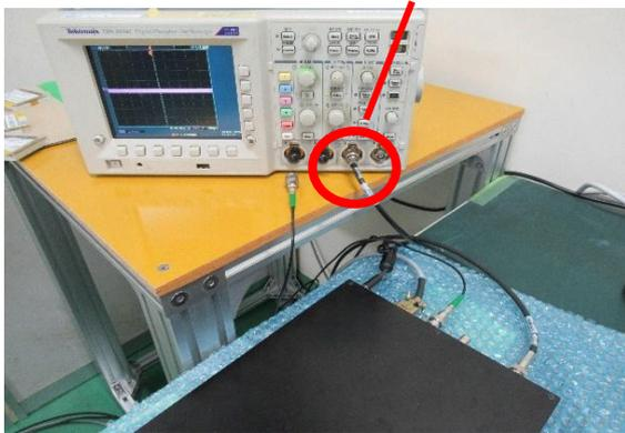
Connect the preamp signal, which is connected to the rear panel (②), to the oscilloscope.
