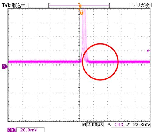
This is the adjustment after setting the "fast pole zero" value to 100 digits in the application, eliminating the undershoot.
