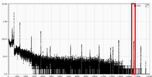
Adjust the "digital coarse gain" and "digital fine gain" to achieve the target of 14550 digits for the 1333 keV peak.
