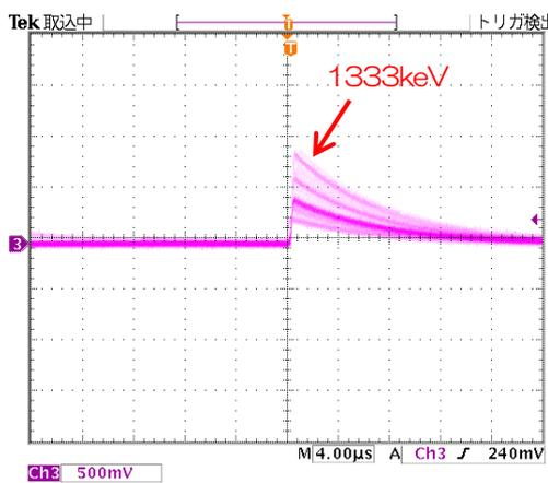
By setting the "analog coarse gain" to x5 and the "analog fine gain" to 222, the waveform of the 1333keV Co-60 signal was adjusted to approximately 880mV, with a clear and well-defined peak.
