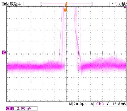
As with the adjustment of the "analog pole zero," the voltage range on the oscilloscope was changed from 20mV to 2mV, and undershoot was observed.
