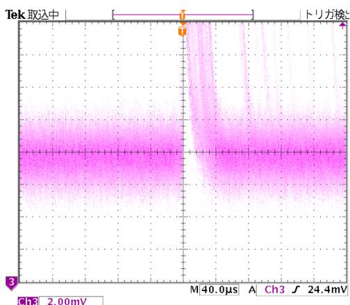
The "analog pole zero" value was adjusted to 183 digits, and the overshoot was completely eliminated.
