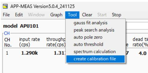
Energy calibration using a quadratic equation requires a calibration file.
